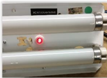
a. Power on L2 only (battery charging)
